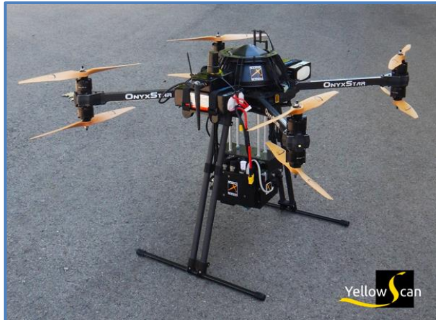
Figure 7. Yellow Scan LIDAR mounted on OnyxStar FOX-C8-HD (sUASnews.com)
