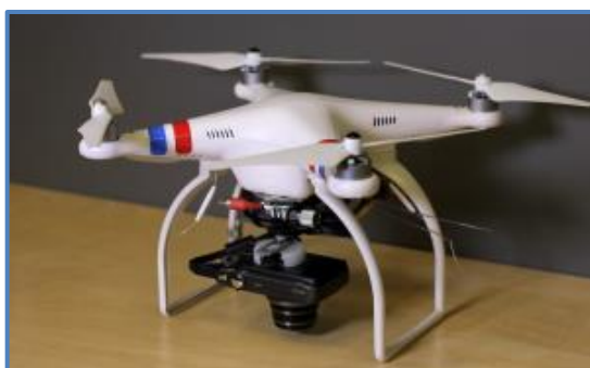
Figure 3. DJI drone with Canon Powershot SX260 (Kreimer and Waite 2014)
